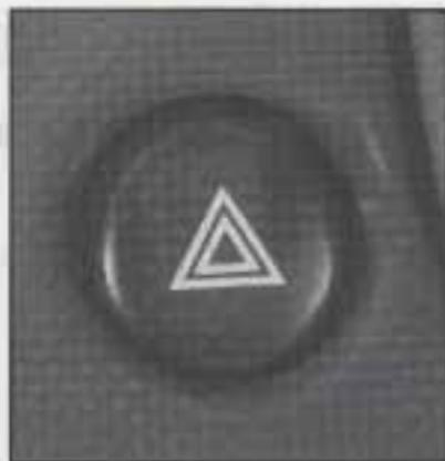
Press the switch once to turn your hazard flashers on. The switch will flash when activated.
