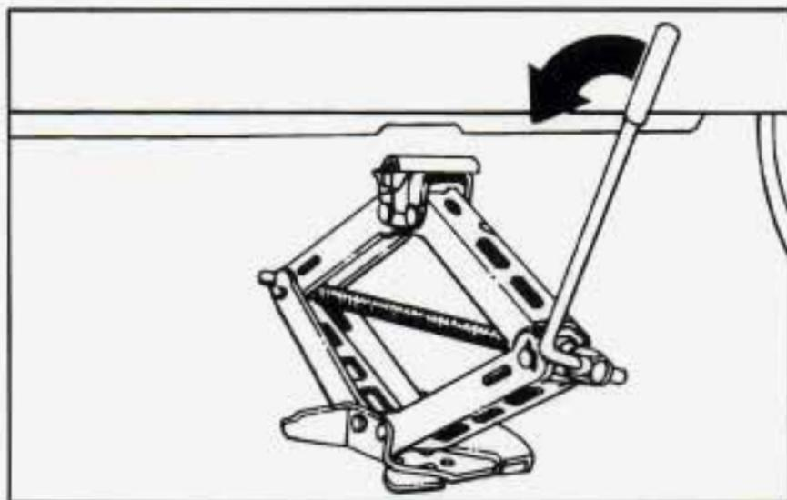
10. Lower the vehicle by turning the wheel wrench to the left. Lower the jack completely.
