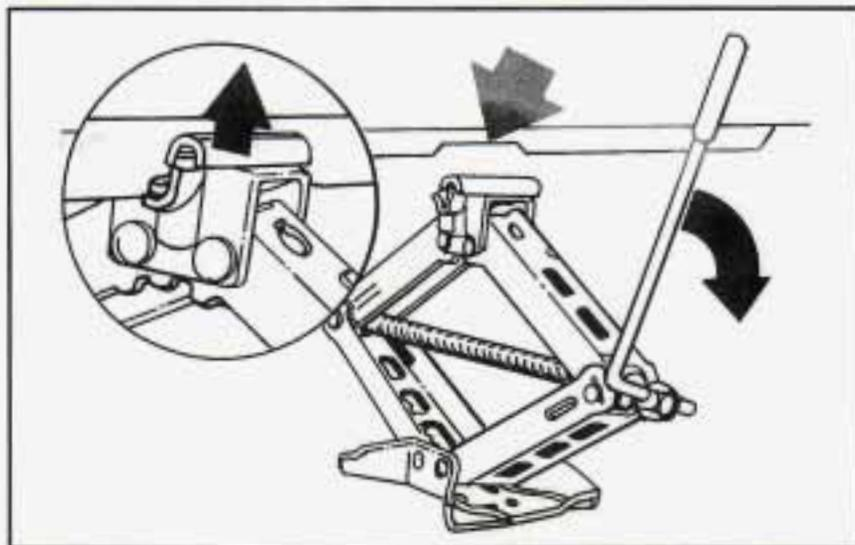
5. Raise the vehicle by turning the wheel wrench to the right. Raise the vehicle far enough off the ground so there is enough room for the spare tire to fit.
