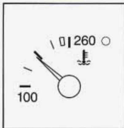
This gage shows the engine coolant temperature. If the gage pointer moves into the red area, the light comes on and you hear a chime, your engine is too hot! It means that your engine coolant has overheated.
