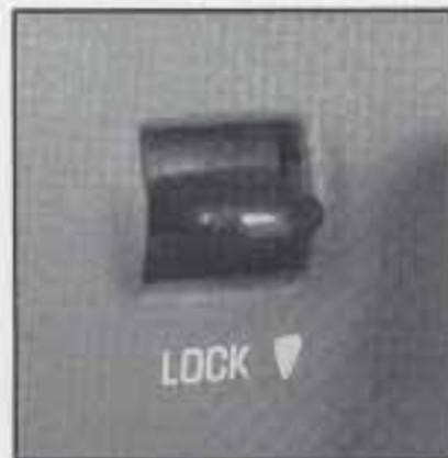
With the power door locks, you can unlock or lock all of the doors of your vehicle from the driver's or front passenger's door lock switch.
