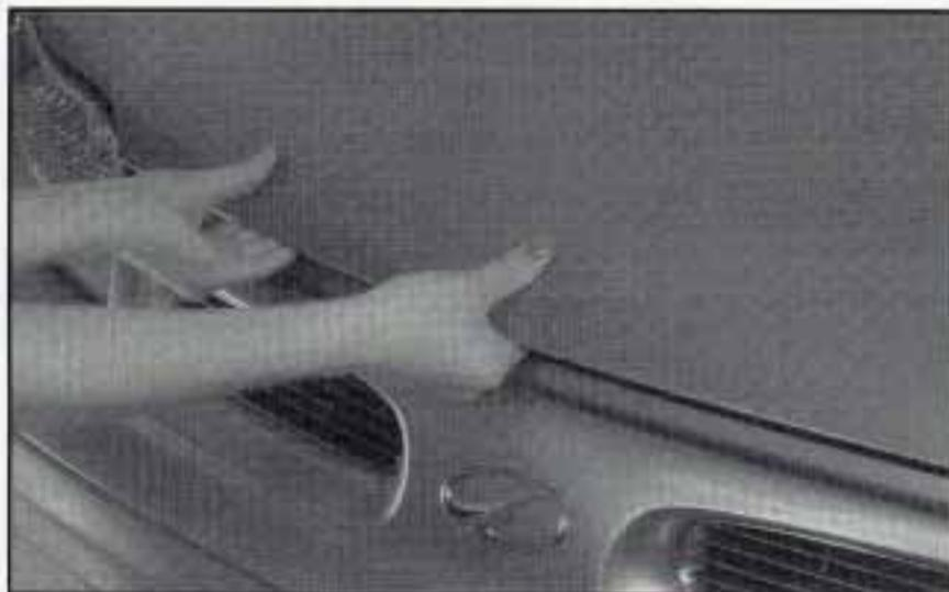
Then go to the front of the vehicle and lift the secondary hood release handle before lifting.
