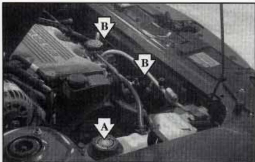
A. Coolant Surge Tank with Pressure Cap
