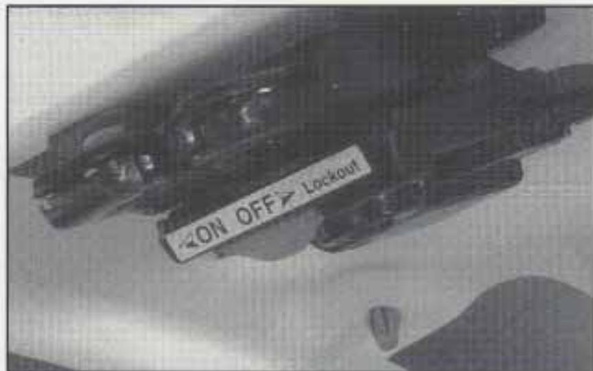
To turn the lockout on, slide the switch all the way to the left. To turn the lockout off, slide the switch all the way to the right.
