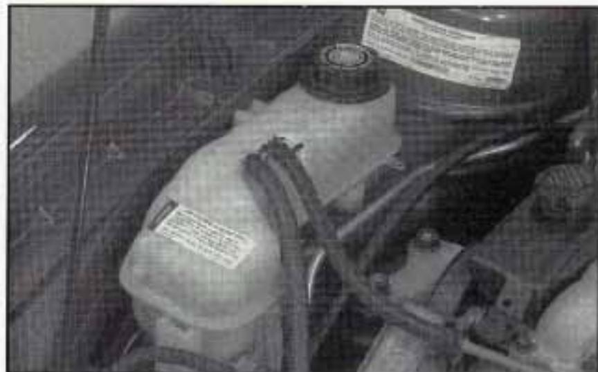
The coolant level should be at or above FULL COLD mark or slightly higher.
