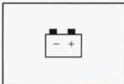
The charging system indicator light will come on when you turn on the ignition, but the engine is not running, as a check to show you it is working.
