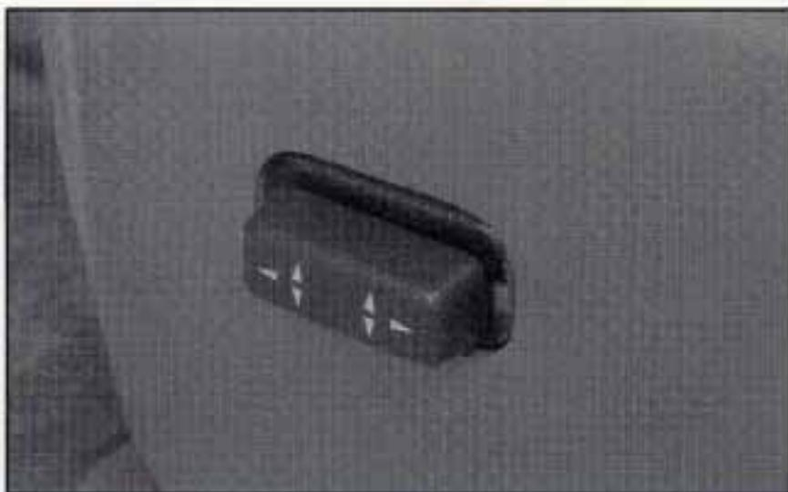
The power seat button is located on the lower, left side of the driver's seat. This button allows you to move the seat up, down, forward and backward. It also moves the front of the seat up or down and the rear of the seat up or down.
