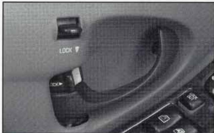
From the inside, to lock the door, move the locking lever forward.
