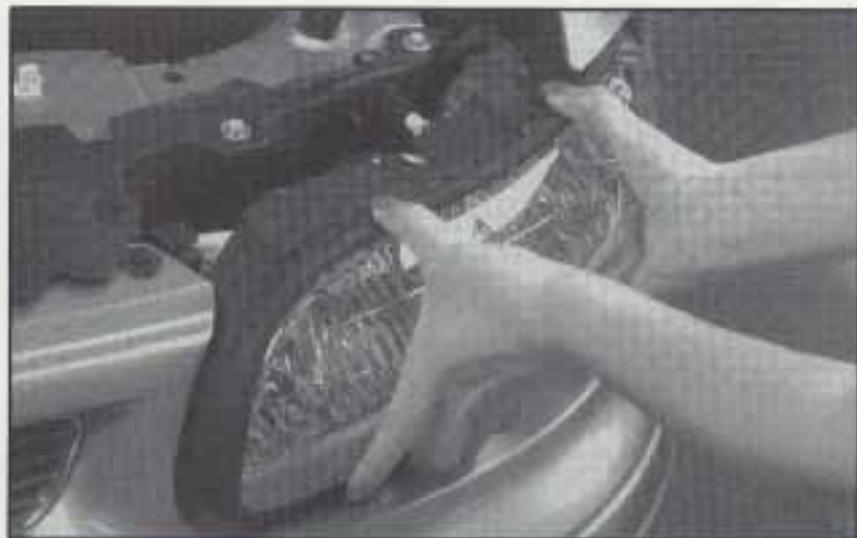
3. Remove the lamp assembly from the vehicle by pulling forward. Use care not to scratch the vehicle with the lamp or the lamp with the fender.
