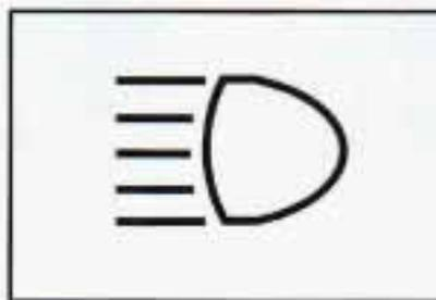
To change the headlamps from low beam to high beam, push forward on the turn signal/multifunction lever.
