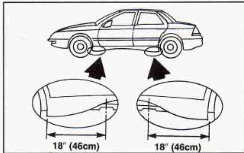
4. Position the jack and raise the jack head until it fits firmly into the notch in the vehicle's frame nearest the flat tire. Put the compact spare tire near you.
