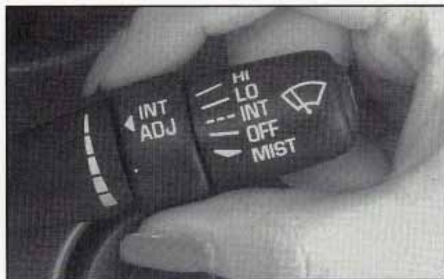
Move the stalk to INT, then rotate the inner band, labeled INT ADJ, and choose the delay you want. Rotate the inner band up for shorter delay times between wiper cycles. Rotate the band down for a longer delay time between wiper cycles.
