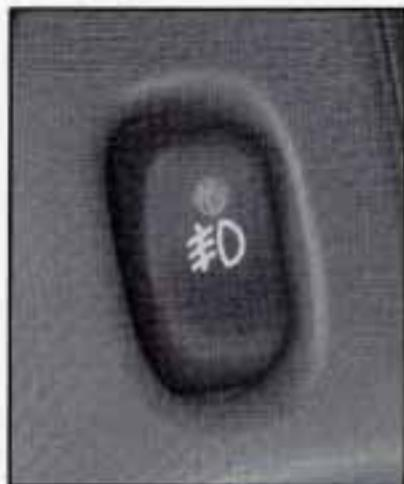
The button for your fog lamps is on the instrument panel, to the left of the steering wheel, beside the instrument panel intensity control.
