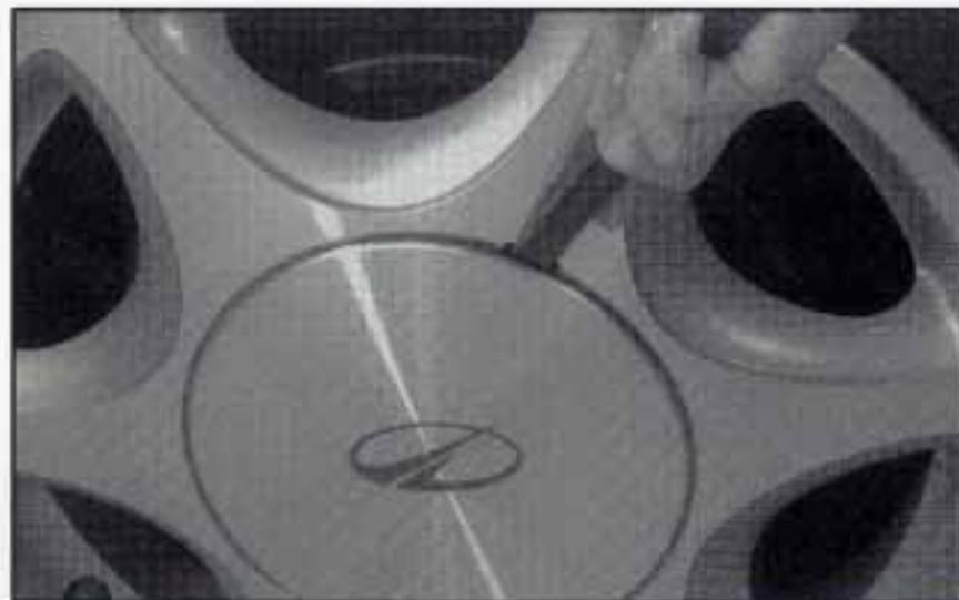
2. Some models are equipped with aluminum wheels. Remove the cover plate to find the wheel nuts. Carefully use the wedge end of the wheel wrench to pry it off.
